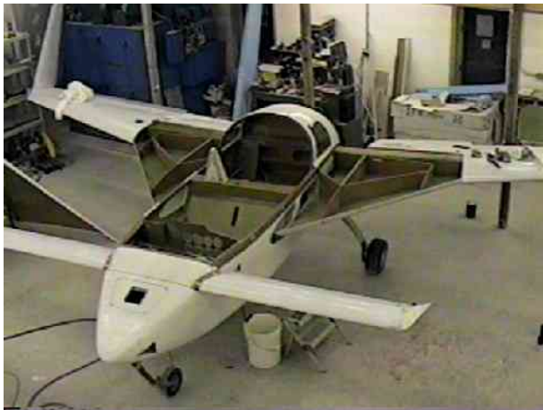
Upper picture of bottom strakes installed with bulkheads in place
