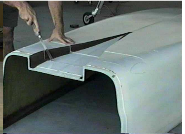
Cutting gear door out of fuselage.
