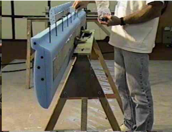
Bonding the trailing edge to the spar.
